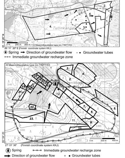
Fig. 2. Locations of the forest stand compartments, groundwater tubes, spring and the immediate groundwater recharge zone in the Lammi area. The number of forest stand compartments refers to Table 1.
