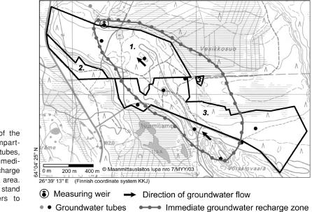
**Fig. 4.** Locations of the forest stand compartments, groundwater tubes, spring and the immediate groundwater recharge zone in the Pyhäntä area. The number of forest stand compartments refers to Table 1.
