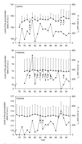
**Fig. 5**. The annual average level of the groundwater table (upper line) and the difference between precipitation and evaporation (P - E) (lower line) at the nearest monitoring station in the Lammi, Valkeala and Pyhäntä areas. F = Final cutting = Clear-cutting or natural regeneration, H = Harrowing, T = Thinning. Standard deviations of the level of the groundwater table are indicated above the lines.
