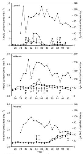
**Fig. 6**. Annual average and maximum nitrate concentrations in groundwater (two lowest lines) and the amount of atmospheric nitrate deposition (uppermost line) at the nearest monitoring station in the Lammi, Valkeala and Pyhäntä areas. F = Final cutting = Clear-cutting or natural regeneration, H = Harrowing, T = Thinning. Standard deviations of the groundwater nitrate concentrations are indicated above the lines.
