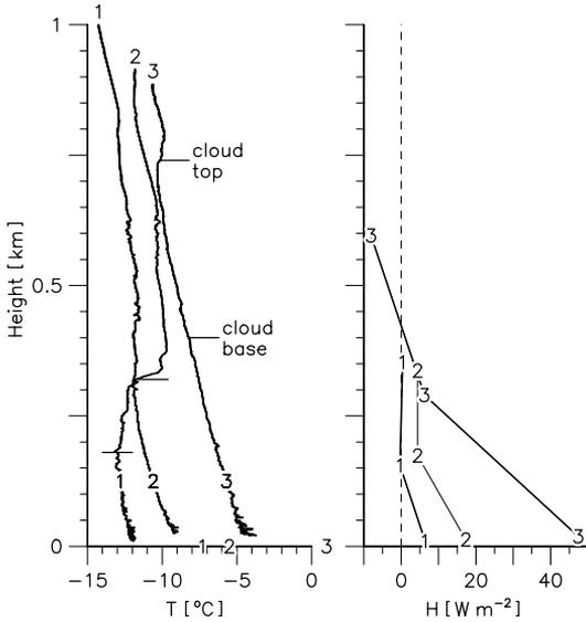
**Fig. 3.** Vertical profiles of temperature ( $T$ ) and sensible heat flux ( $H$ ) over sea ice at  $\Delta x = -130$  km (1) and  $\Delta x = -40$  km (2) distance from the ice edge and over water at  $\Delta x = 40$  km (3). Surface temperatures are marked by respective numbers. There were no clouds at (1) and (2) and 6–8 octas stratocumulus between 400 and 750 m at (3). Horizontal bars indicate boundary layer top or cloud layer boundaries, respectively.
