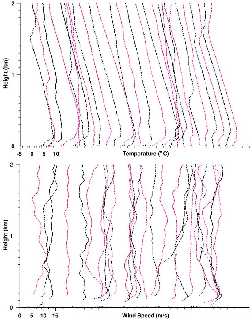
**Fig. 7.** Six-hourly profiles of temperature (above) and wind speed (below) measured by radiosondes launched on board of *Alkor* at 56°N, 18.5°E during 4 April 00 UTC and 10 April 2001 06 UTC. The running abscissa scale marks the 10 °C temperature value and the 15 m s<sup>-1</sup> wind speed value, respectively.
