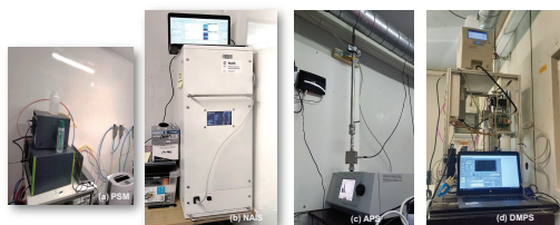
Fig. 5. Aerosol measurement instruments: (a) NAIS installed in AL-1; (b) PSM installed in AL-2; (c) APS installed in AL-3; and (d) DMPS installed in AL-3.
