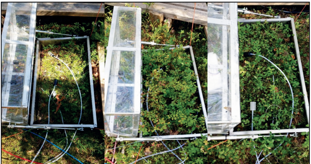
Fig. A1_1. Soil chambers (10, 13 and 15 respectively) used during the sampling campaign.
