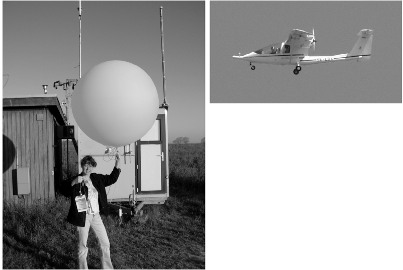
Fig. 2. Pictures from the RIMI site during the experiment. Left-hand picture shows a launch of a radiosonde and the right-hand picture the airplane performing measurements.
