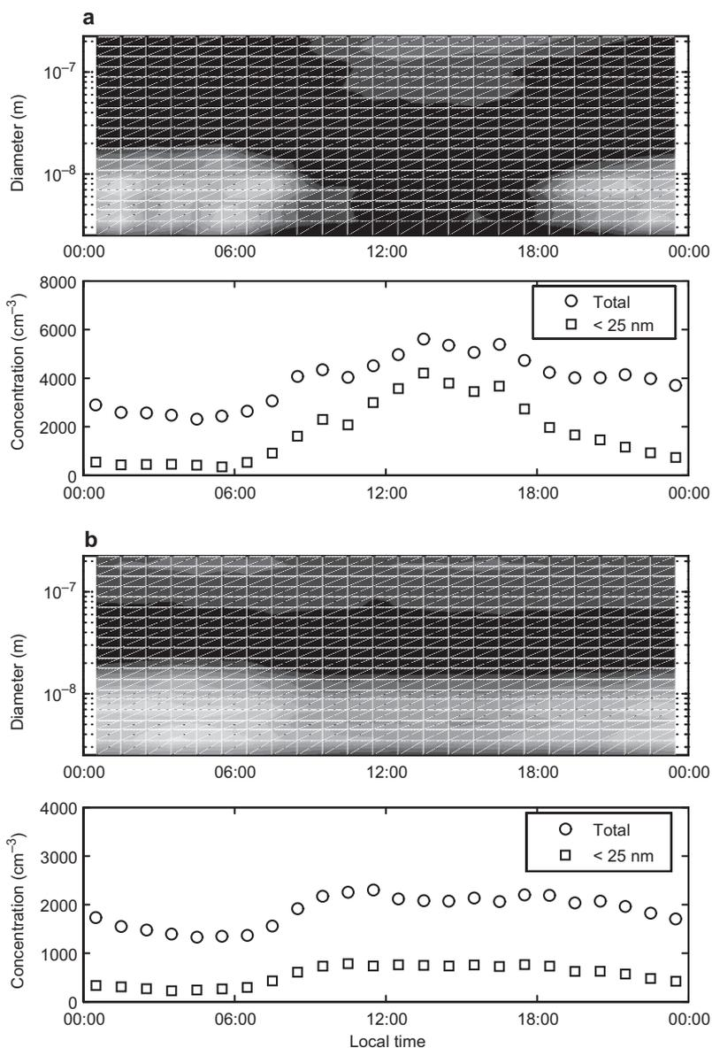
**Fig. 5.** The average diurnal evolution of the measured size distributions and total number concentrations at the Tomsk measuring station on (a) event and (b) non-event days. Note that the size distributions were restored from integral characteristics and are thus approximations of the real size distributions.
