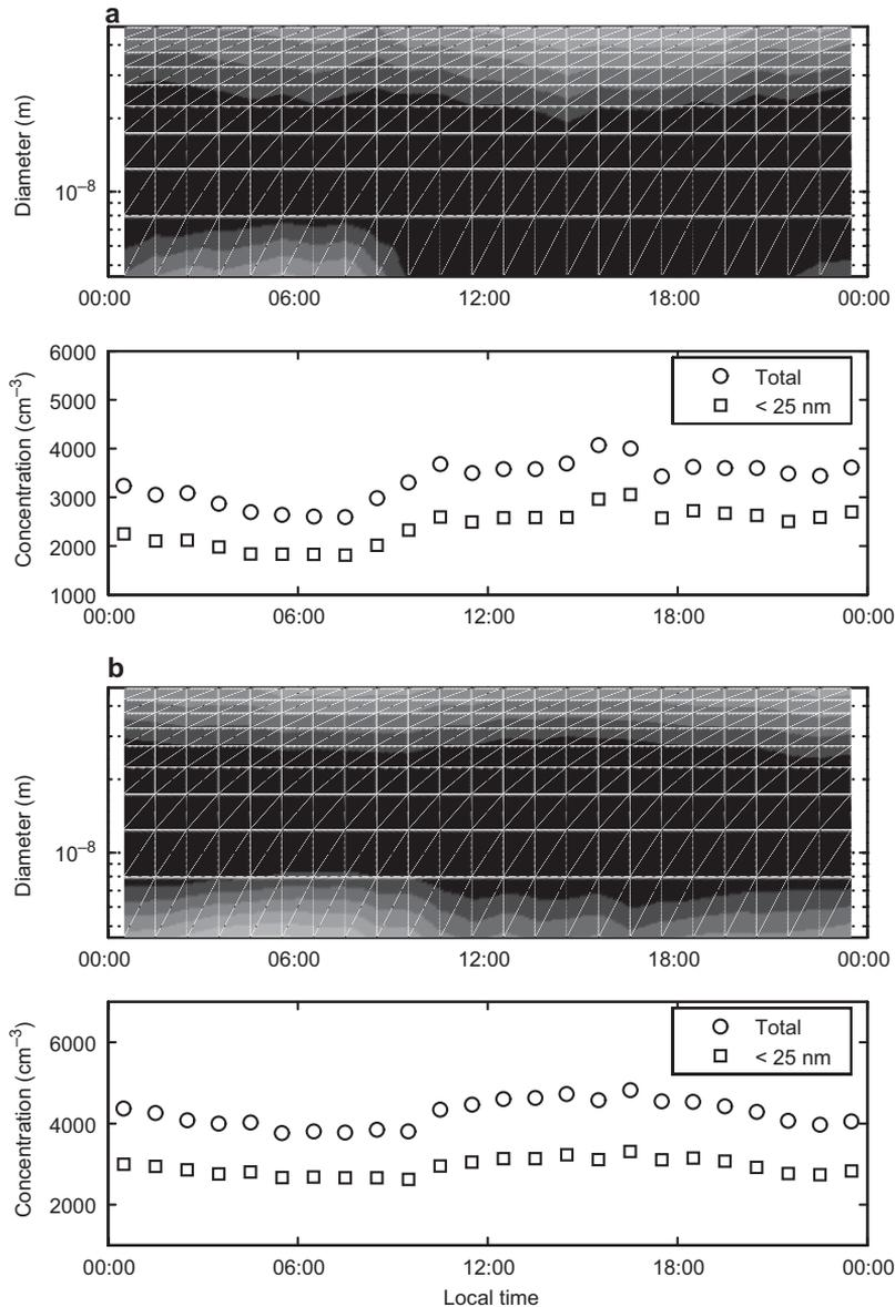
**Fig. 6.** The average diurnal evolution of the measured size distributions and total number concentrations at the Listvyanka measuring station on (a) event days and (b) all other days. Note that the size distributions were restored from integral characteristics and are thus approximations of the real size distributions.
