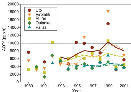
**Fig. 7.** Values of the AOT40 exposure index for forests (April–September) at the Finnish EMEP and GAW sites. The 5-year averages and the corresponding critical level of 10 000 ppb h are also indicated.
