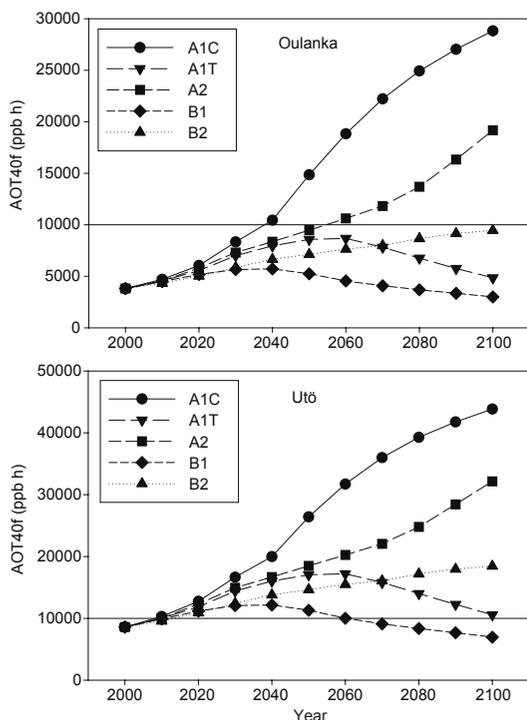
**Fig. 10.** Modelled development of AOT40f at Oulanka and Utö for different SRES scenarios. The critical level of 10 000 ppb h is also indicated.
