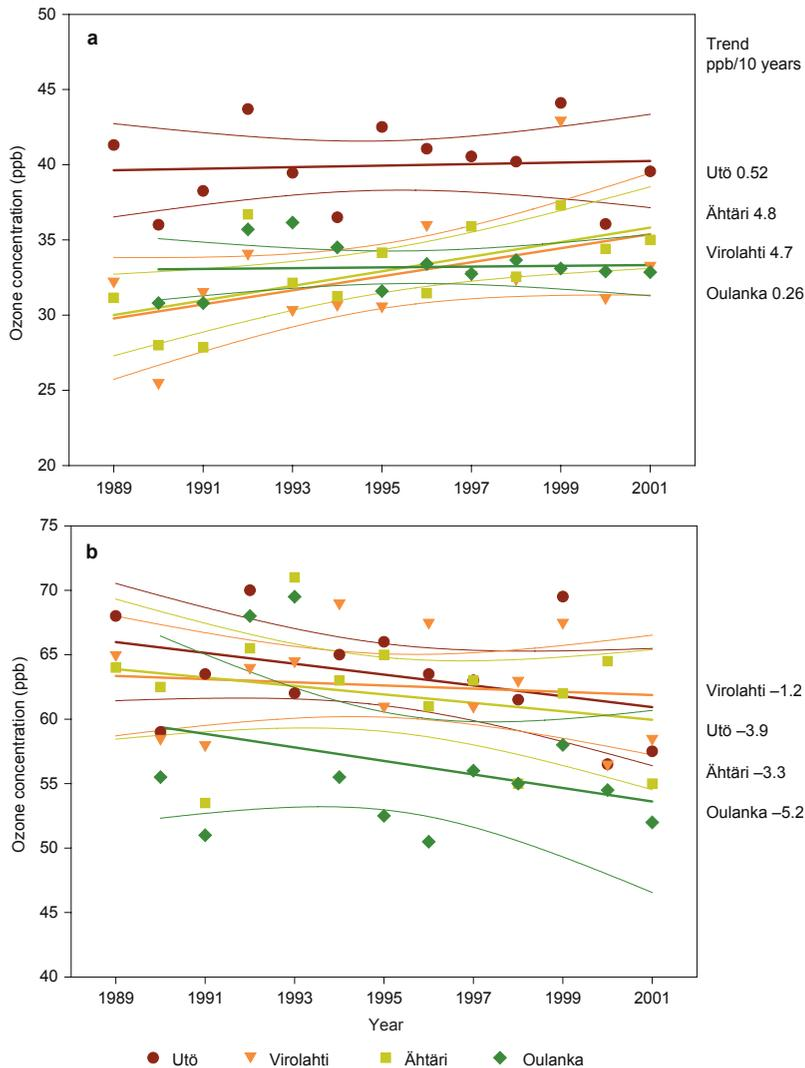
**Fig. 5.** Averages (a) and the 99th percentiles (b) of hourly daytime ozone concentrations in May–July. Linear regressions together with the 95% confidence intervals are also shown. Trend estimates are based on the linear regression and are not significant at  $p < 0.1$  level.
