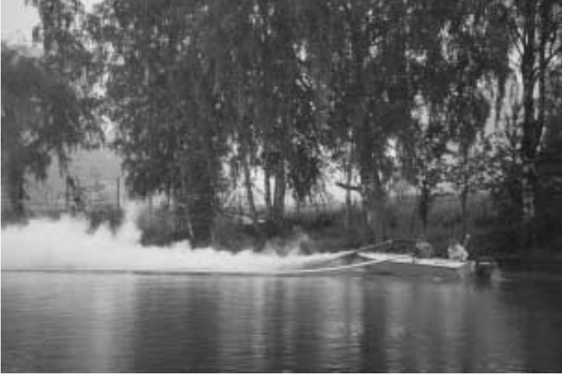
Fig. 2. A motor boat was used to distribute the gypsum through the lake water to sediments of Lake Laikkalammi.
