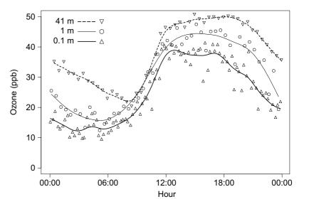
**Fig. 3.** Concentration of  $O_3$  (ppb v/v) during 25 May 2002 in three heights (0.1 m, 1 m and 41 m). Points are measurements averaged over 1 min after a stabilization time to each height of 2 min; lines are smoothed splines.
