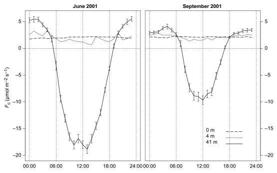
**Fig. 4.** Mean monthly diurnal variation in fluxes of  $CO_2$  ( $F_c$ ) during June and September 2001 measured above canopy and in trunkspace by eddy covariance and at soil surface by dynamic chambers. Bars denote ± standard error of the mean.
