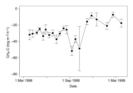
Fig. 5. Fluxes of methane measured in soil chambers over the course of one year from March 1998 to March 1999. Points are means of six replicate chambers and bars show ± standard errors of the mean.
