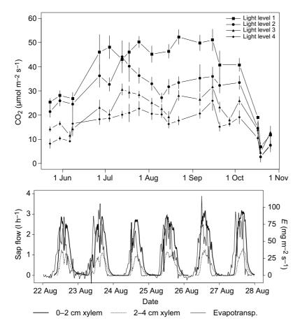
Fig. 9. Seasonal photosynthesis ( $A_{max}$ ) in four canopy layers at constant levels of temperature (20 °C), CO<sub>2</sub> (1800 ppm) and PAR (1500 µmol m<sup>-2</sup> s<sup>-1</sup>).
