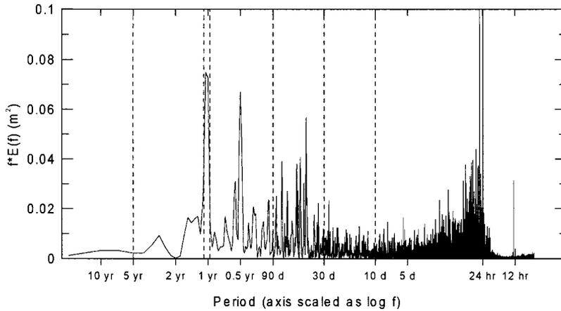
**Fig. 6.** Sea level power spectrum, calculated with a Blackman-Harris window, from the detrended time series of the 4-hour interval values at Helsinki, years 1980–1999. The annual and semiannual cycles are visible, as well as the diurnal and semidiurnal tidal components. The two diurnal tides visible extend beyond the axis limits. (The 25.8 h component extends to  $0.71 \text{ m}^2$  and the 23.9 h component to  $0.74 \text{ m}^2$ .)
