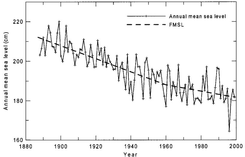
**Fig. 9.** Annual mean and fitted mean sea level (FMSL) at Hanko, referred to the FIMR standard bedrock-bound reference level.
