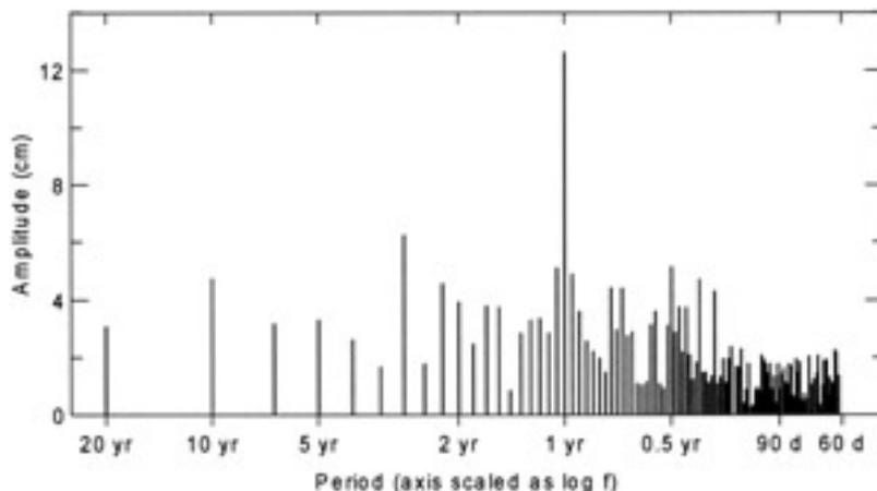
**Fig. 7.** Sea level amplitude spectrum, calculated from the detrended time series of the monthly means at Helsinki, years 1980–1999. The annual cycle is distinctly visible.
