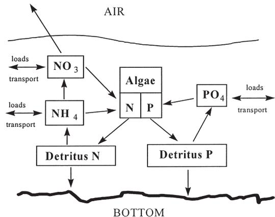
Fig. 2. Flowdiagram of nutrients modelled by FINNALGA.
