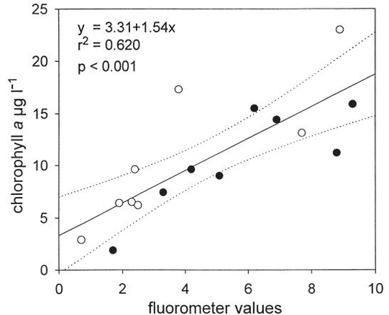
**Fig. 4.** The correlation between fluorometer values and chlorophyll *a* content in Lake Ladoga in the year 1995. Open dot = all sampling stations in 1995, black dot = sampling stations, where light transmission has been measured. Broken lines denote the 95% confidence belt.
