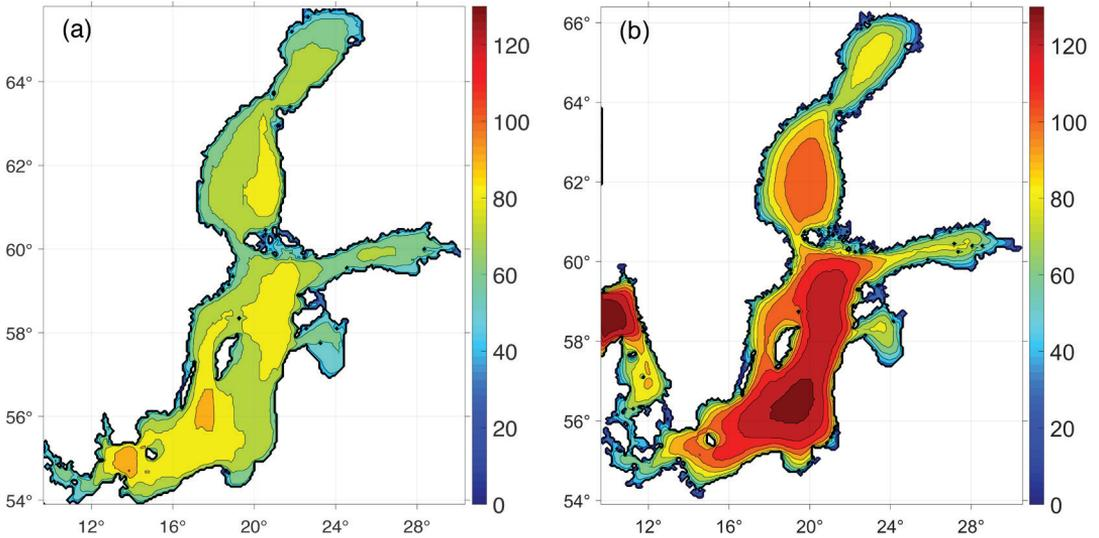
**Fig 2.** Long-term average significant wave height (cm) in the Baltic Sea from 1970–2007 from the WAM model forced by (a) geostrophic winds (adapted from Räämet and Soomere 2010) and (b) COSMO winds.
