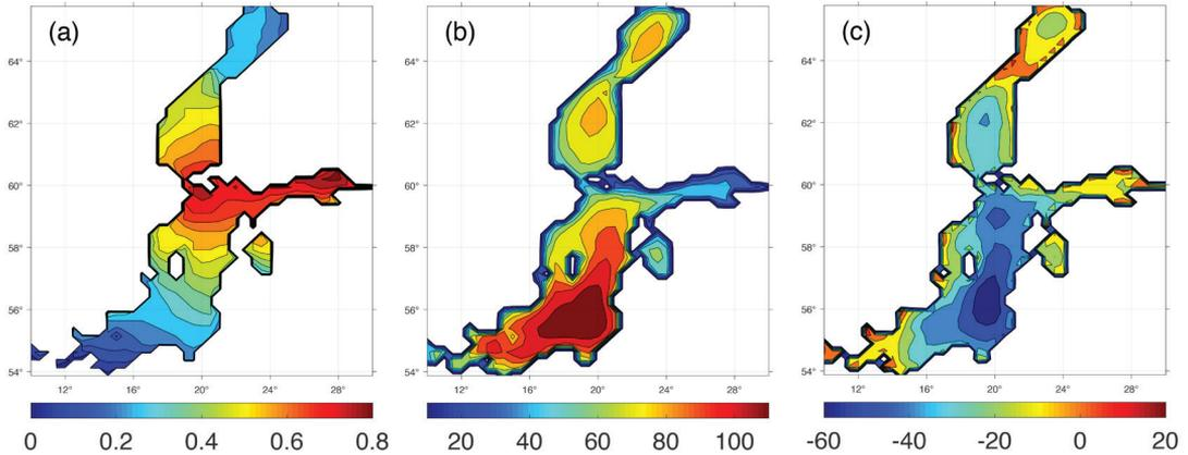
**Fig 3.** (a) Correlation, (b) root mean square deviation and (c) bias (cm) between modelled wave data produced by models forced using geostrophic winds and COSMO winds. Negative bias means that the model forced by COSMO winds gives higher waves than the model driven by geostrophic winds.
