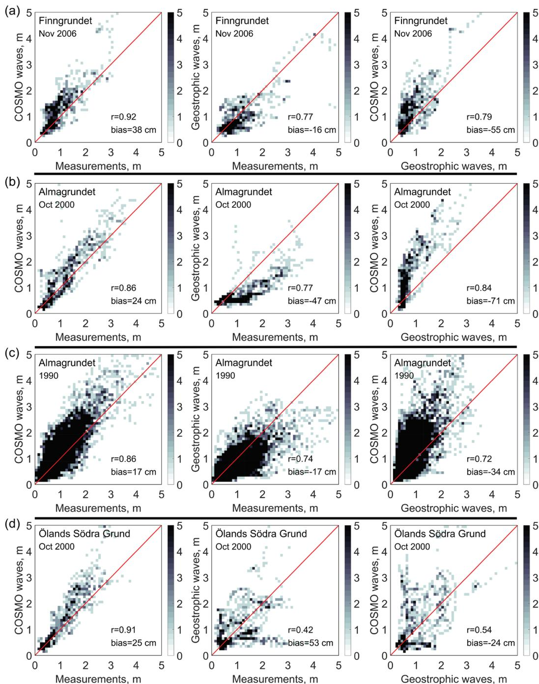
**Fig 5.** Scatter plot of measured and modelled significant wave heights at the locations of the SMHI wave buoys. The brightness scale shows the number of wave events in pixels with dimensions of 10x10 cm. Panels (a), (b) and (d) represent single windy months whereas panel (c) represents one year.
