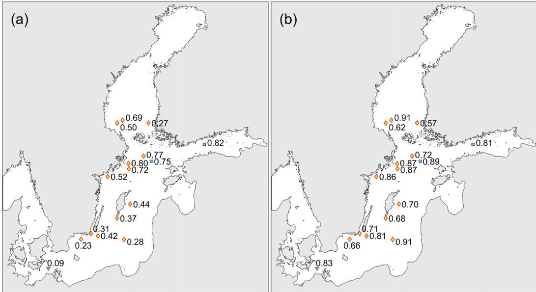
**Fig 4.** Correlation coefficients between measured wave properties at the locations of the SMHI, FMI and ICR measurement sites and wave heights simulated using (a) geostrophic winds and (b) COSMO winds.
