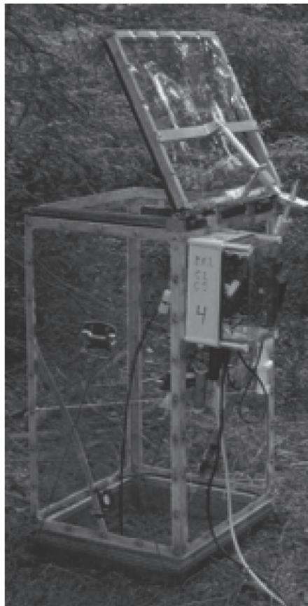
**Fig 3.** One of six automatic chambers used to measure CO<sub>2</sub> fluxes.
