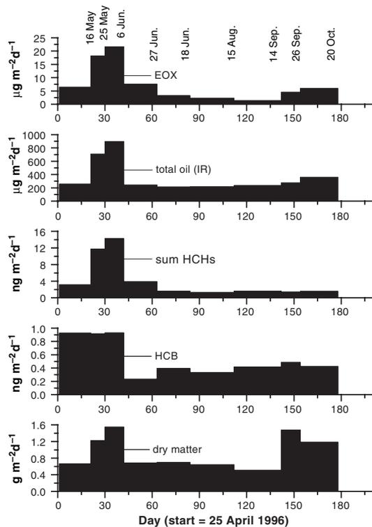
**Fig. 7.** Sedimentation of EOX ( $\mu\text{g Cl m}^{-2} \text{d}^{-1}$ ), total oil ( $\mu\text{g m}^{-2} \text{d}^{-1}$ ), HCHs ( $\text{ng m}^{-2} \text{d}^{-1}$ ), HCB ( $\text{ng m}^{-2} \text{d}^{-1}$ ), and dry matter ( $\text{g m}^{-2} \text{d}^{-1}$ ) to the automatic trap at station GF2 during the experiment (25 April–20 October 1996).
