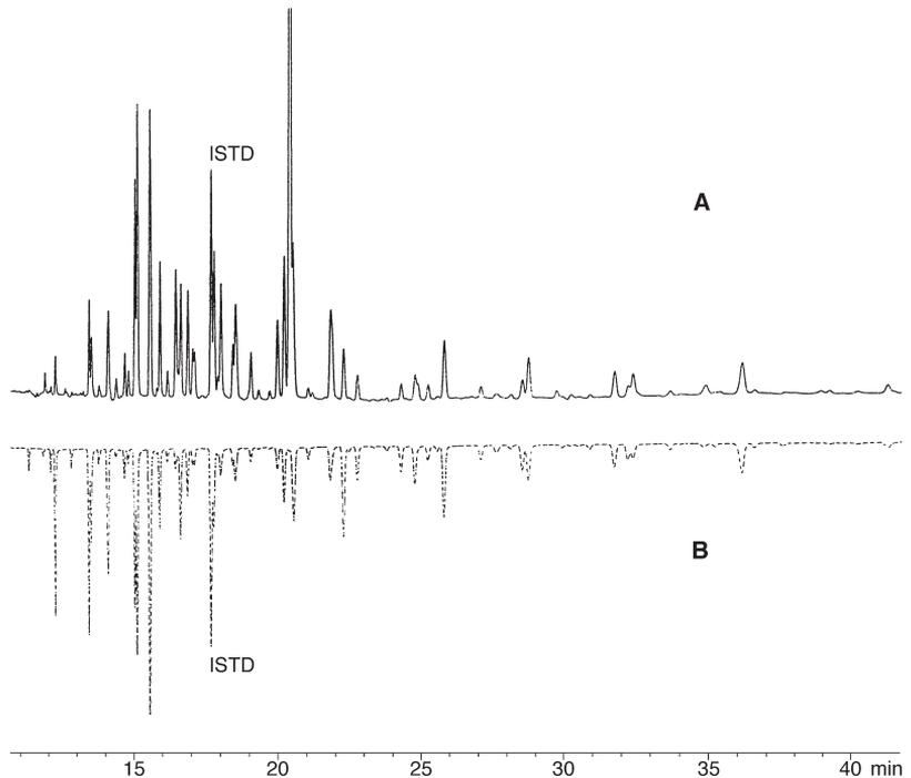
**Fig. 9.** Mirrored ECD-chromatograms (column HP-5) of the Schepelev trap sample (A) and a mixture of Pyralene 3010 and Clophen A50 in relative concentrations 2:1 (B). ISTD = internal standard. Chromatographic conditions are given in the material and methods section.
