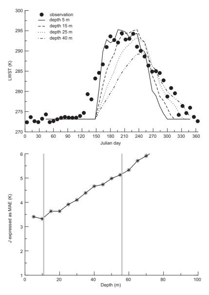
lake LWST simulations with four different lake depths, viz., 5 m, 15 m, 25 m, and 40 m for Lake Konnevesi (no. 4 in Table 1). In the upper panel, lines show simulation results, and circles show observations. The lower panel shows the cost function for different lake depths based on the LWST Mean Absolute Error (MAE). The vertical lines indicate mean and maximum lake depths, respectively, based on in situ measurements
