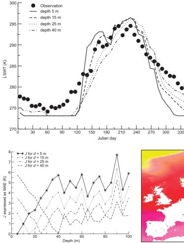
**Fig. 2.** Cost function *J* expressed as Mean Absolute Error (MAE) between the model LWST and the simulated LWST observations for Lake Vanern (no. 43 in Table 1). Simulated LWST observations are generated assuming a "true" lake depth of 5, 15, 25 and 40 m (consistently with Fig. 1). The existence of a single minimum of the cost function coincident with the "true" lake depth is verified for all four depths considered.
