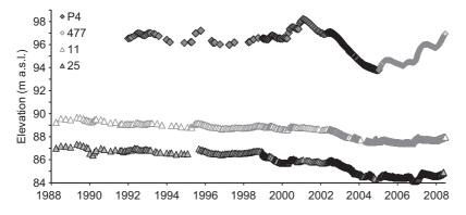
Fig. 2. Hydraulic heads of the selected groundwater monitoring wells. Wells P4 and 477 are located in the Kankaanjärvi perched aquifer. Wells 11 and 25 represent the hydraulic head changes in the main aquifer hosted by glaciofluvial deposits (units 2 and 3).
