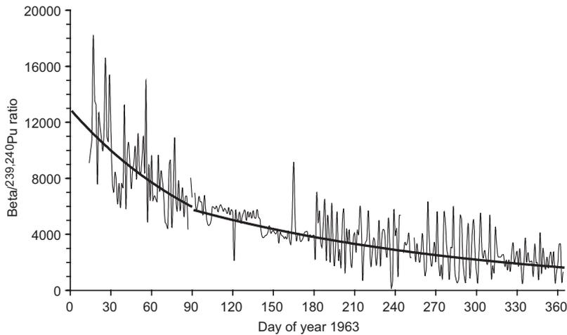
**Fig. 8.** The ratio of total beta activity to  $^{239,240}\text{Pu}$  activity concentration in the air of Sodankylä in 1963.
