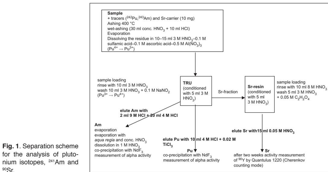
**Fig. 1.** Separation scheme for the analysis of plutonium isotopes,  $^{241}\text{Am}$  and  $^{90}\text{Sr}$ .
