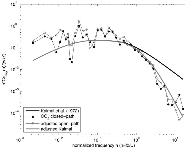
**Fig. 4.** The frequency behavior of a closed-path  $\text{CO}_2$  cospectrum can be achieved by multiplying an open-path, or model cospectrum with a transfer function TF (Eq. 5).
