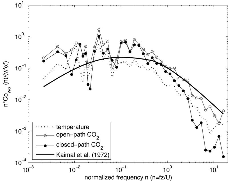
**Fig. 3.** Typical sub-canopy cospectra of vertical wind and temperature and vertical wind and  $\text{CO}_2$  measured with a closed-path and an open-path. Closed-path cospectrum attenuates at frequencies  $n > 2$  relative to open-path and temperature cospectra. A cospectral model (Kaimal *et al.* 1972) shown as a reference.
