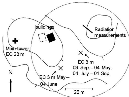
**Fig. 1.** Measurement site and the location of different measurements. The flux footprint area (80%) for trunk-space fluxes is within the large circle. Interval of the contour lines is two meters. EC refers to eddy covariance measurements at respective height.
