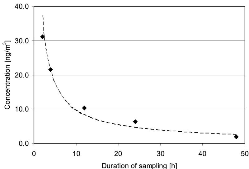
**Fig. 4.** Mean total concentration of even *n*-alkanes ( $C_{12}$ – $C_{28}$ ) measured in aerosol samples collected in 2, 4, 12, 24 and 48-hour periods at Hyytiälä, Finland, in March–April 2003.
