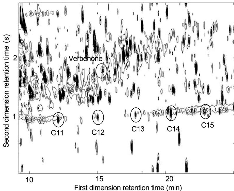
**Fig. 1.** Part of the GC×GC contour plot of an aerosol sample collected at Hyytiälä, Finland, on 10 April, 2003. In the first dimension, the compounds are separated mainly according to their volatility (decreasing to the right) and in the second dimension according to their polarity (increasing upwards). The intensity of the dots increases with the concentration of the compounds. *n*-Alkanes (C<sub>11</sub>–C<sub>15</sub>) and verbenone are marked on the plot.
